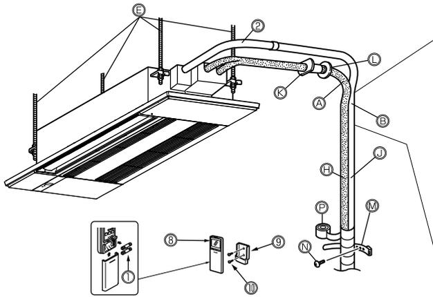
Be sure to use wall hole sleeve ⑫ to prevent indoor/outdoor connecting wire ⑩ from contacting metal parts in the wall and to prevent damage by rodents in case the wall is hollow.
