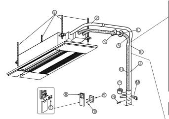
Be sure to use wall hole sleeve ( to prevent indoor/outdoor connecting wire (1) from contacting metal parts in the wall and to prevent damage by rodents in case the wall is hollow.
