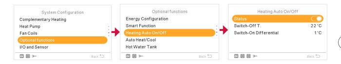
The system computes the 24-hour average outdoor temperature. No evaluations are made within the initial 24 hours. Subsequently, the system dynamically refines this average by incorporating a new temperature sample every 5 minutes, continuously monitoring and adjusting to current conditions.
