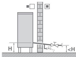
When water is idle inside the system, freezing up is very likely to happen which could damage the system.
