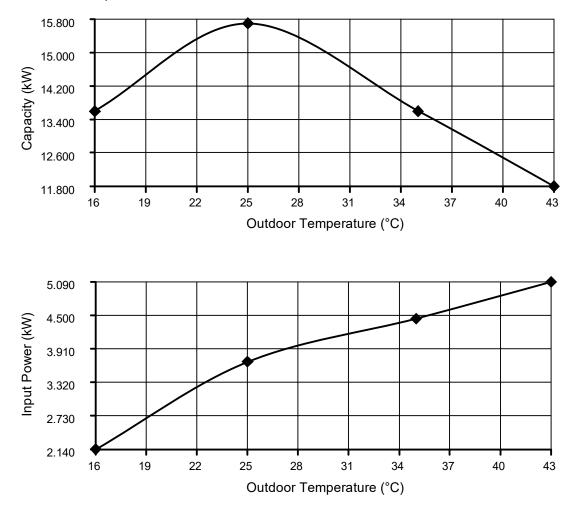
Condition Outdoor air temperature : 35°C (DBT), -°C (WBT) Indoor water inlet temperature : 23°C Indoor water outlet temperature : 18°C
