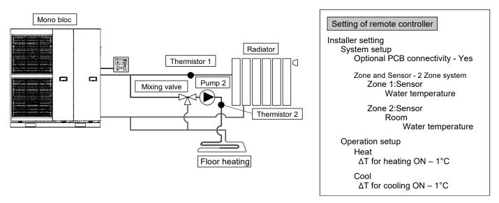
This is an example of simple 2 zone control without using buffer tank.
