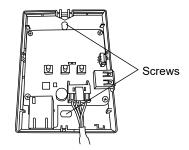
4. Pull the CN-CNT cable through the hole in the bottom of the adaptor and re-attach the front cover to the back cover.
