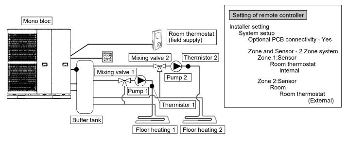
Connect floor heating to 2 circuits through buffer tank as shown in the figure.
