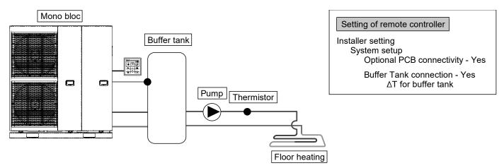
This is an application that connects the buffer tank to the Mono bloc.
