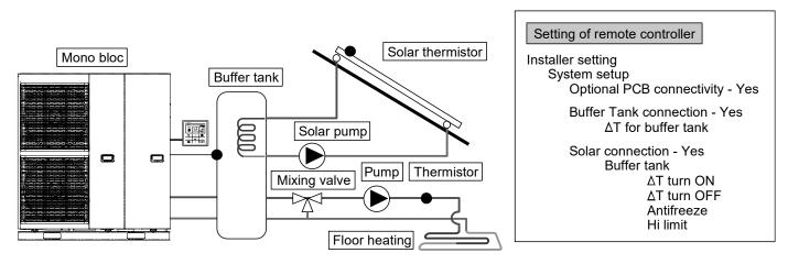
This is an application that connects the buffer tank to the Mono bloc before connecting to the solar water heater to heat up the tank.
