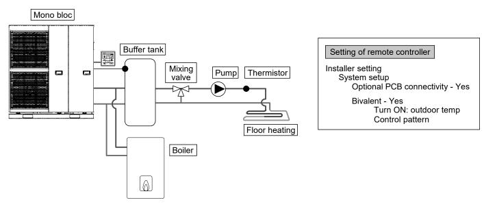
This is an application that connects the boiler to the Mono bloc, to compensate for insufficient capacity by operate boiler when outdoor temperature drops & heat pump capacity is insufficient.
