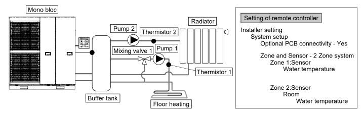
Connect floor heating or radiator to 2 circuits through buffer tank as shown in figure.
