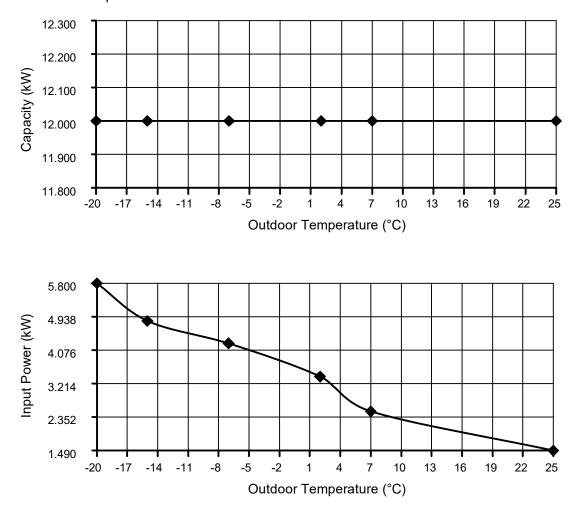
Condition Outdoor air temperature : 35°C (DBT), -°C (WBT) Indoor water inlet temperature : 12°C Indoor water outlet temperature : 7°C
