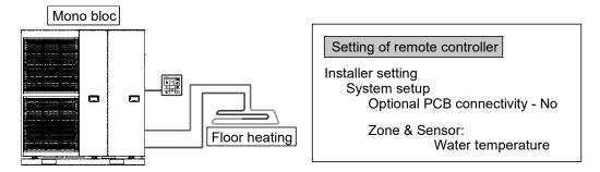
Connect floor heating or radiator directly to the Mono bloc. This is the basic form of the most simple system.
