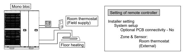
Connect floor heating or radiator directly to Mono bloc.
