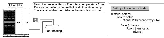
Connect floor heating or radiator directly to the Mono bloc. Install the remote controller in the room where floor heating is installed. This is an application that uses remote controller as Room Thermostat.
