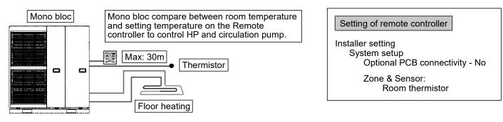
Connect floor heating or radiator directly to Mono bloc. Install separate external room thermistor (specified by Panasonic) in the room where floor heating is installed. This is an application that uses external room thermistor.
