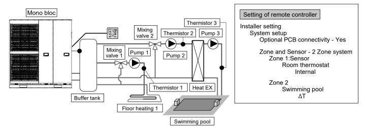
Connect floor heating and swimming pool to 2 circuits through buffer tank as shown in figure.
