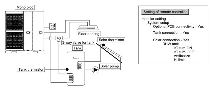
This is an application that connects the DHW tank to the Mono bloc through 3-way valve before connect the solar water heater to heat up the tank. DHW tank's temperature is detected by tank thermistor (specified by Panasonic). Solar panel's temperature is detected by solar thermistor (specified by Panasonic).
