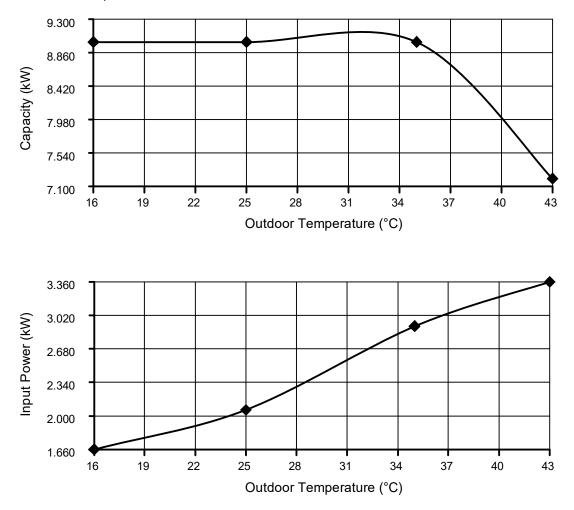
Condition Outdoor air temperature : 35°C (DBT), -°C (WBT) Indoor water inlet temperature : 19°C Indoor water outlet temperature : 14°C
